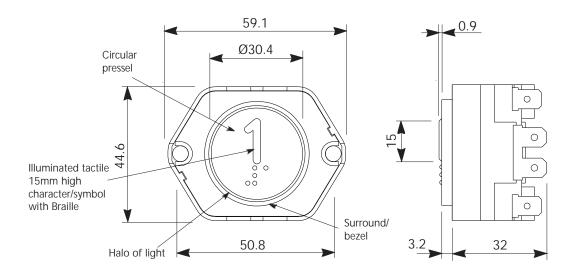
Compact 2 Pushbuttons can be supplied loose or incorporated into stations with 1.5mm or 2.5mm stainless steel faceplates, with a vertical pitch of 50mm and horizontal pitch of 60mm i.e the pushbutton body can be rotated through 90 degrees (horizontal version shown above). If pushbuttons are supplied loose, spacers are provided to accommodate the differing faceplate thickness.
